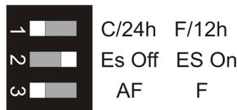
Figure 3: TH115-AF Thermostat DIP Switches
